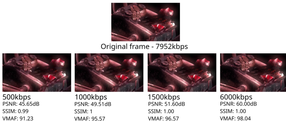
Figure 6: ED metrics on still scene from 500kbps to original with a factor 5 zoom.
